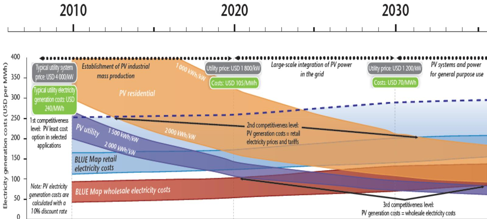
LCOE<sub>PV</sub> Source: IEA, PV Technology road map, oct2010
